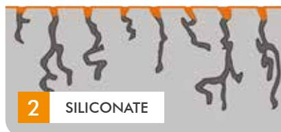
The siliconate in EUCO Diamond Hard also reacts to create a liquid-repellent seal on the concrete surface.
