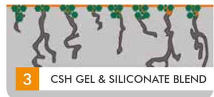
The synergistic activity of the silicate & siliconate blend in EUCO Diamond Hard seals and strengthens the concrete.
